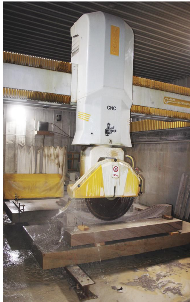
Additionally, a Gmm 6-axis CNC bridge saw is used to cut stone pieces.
