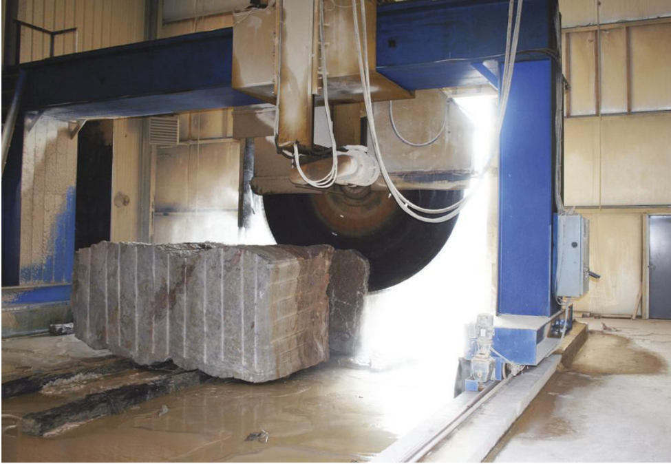
Blocks are first cut into slabs with either a Park Industries Eagle or Wilson saw.
