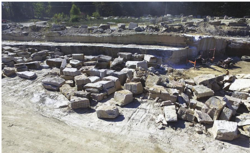
"The average size of the blocks extracted at the quarry are 5 x 10 x 40 feet. "They are then sized to 5 x 5 x 12 feet before going to the shops," said Dave Curulla of Russell Stone Products, Inc.
