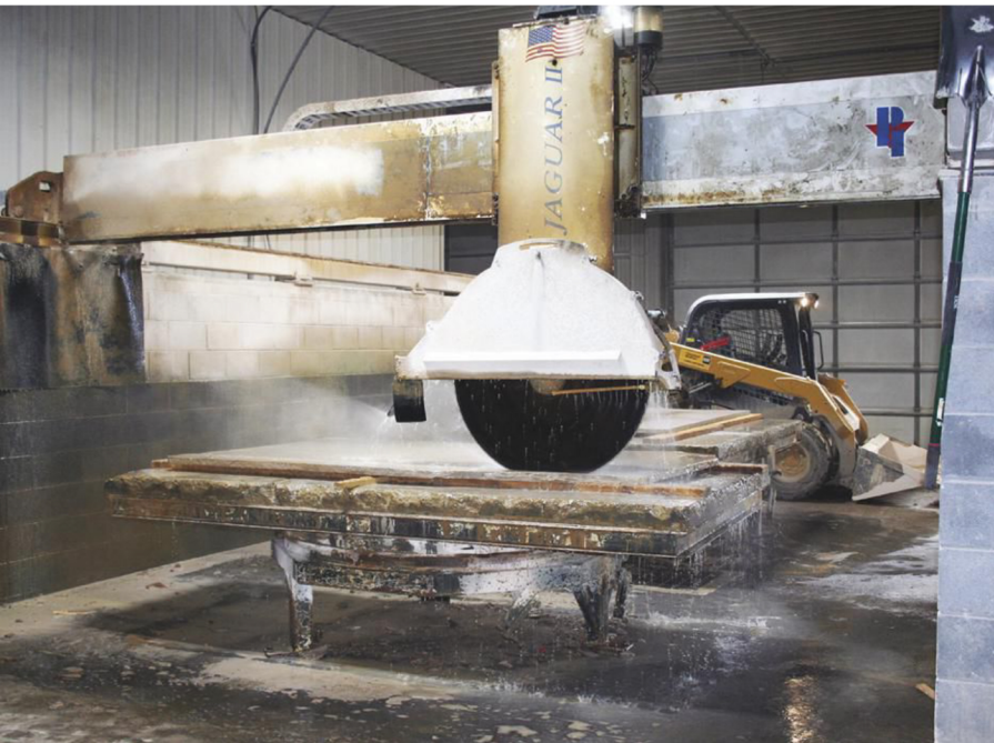
A Jaguar II bridge saw is also on hand in the shop to assist in the fabrication process.
