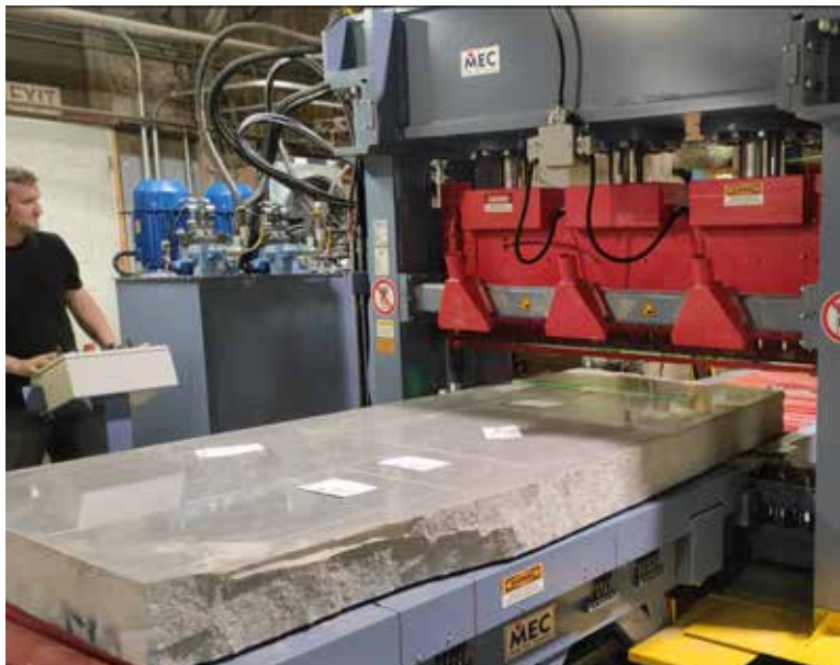
Tesmo H-frame Split-Face splitter for wide full slabs.
