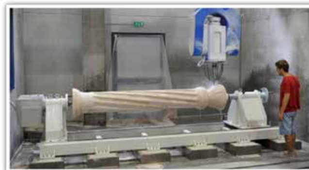
Lathe: interpolated lathe to produce columns of different sizes and complex forms
